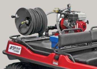
Fire fighting skid unit equipped with Scotty foam system
