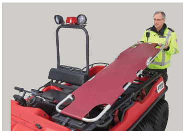
Stretcher mounting kit, stretcher, fold down light bar with beacon and two LED spotlights
