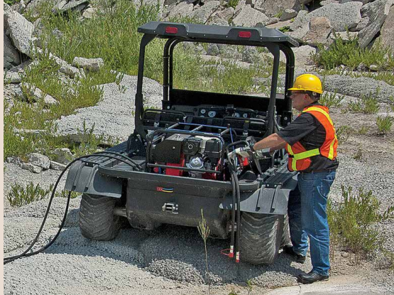
The ARGO Universal Mounting System lets you install external power sources like a hydraulic power pack, generator or compressor increasing the utilization and versatility of your vehicle.
