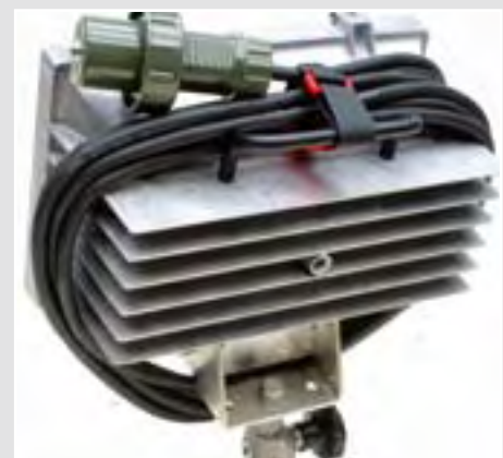
The handle also makes it possible to safely roll up the cable
