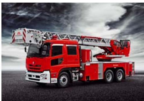
/ Magirus turntable ladder on Hino chassis with 3 axles, three axles steering
