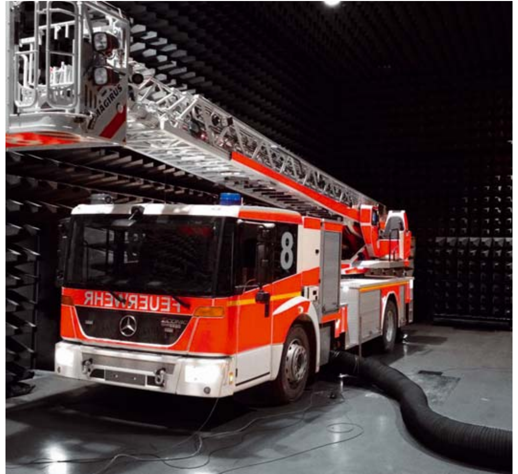
/ Ladder in EMC test
