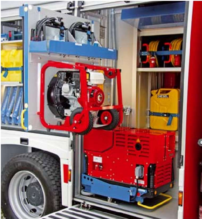
/ Optimum utilisation of space, including depth: The equipment lockers are positioned deep around the axles and offer a third level of storage for secondary materials.
