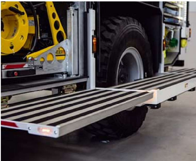
/ The superstructure has no-slip hatches which are stable up to 250 kg. Safe equipment removal is even possible for vehicles with larger tyres.
