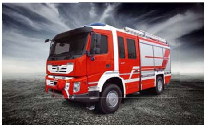
/ Tank pumper 4000 on Volvo 4x4, with MAGIRUS crew compartment in aluminium technology
