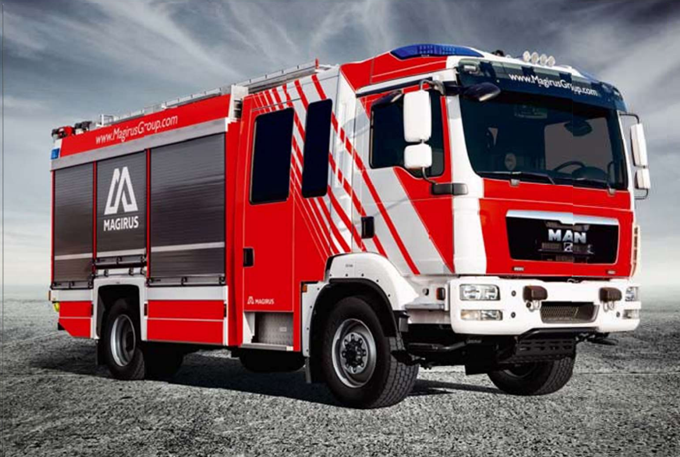
/ 2000 litre class fire-fighting vehicle on MAN 4x4, with MAGIRUS crew compartment in aluminium technology
