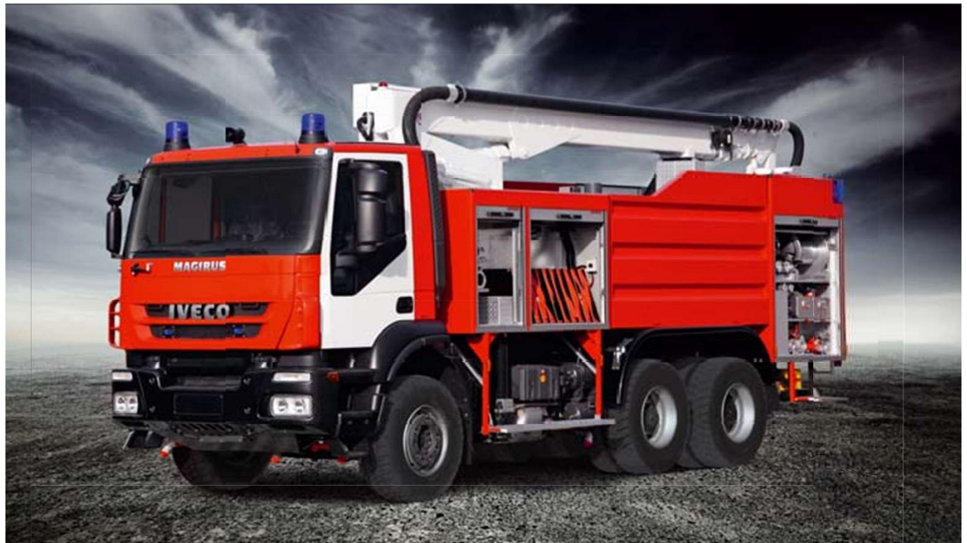
/ Telescopic extinguishing booms enhance the vehicle's tactical abilities for fire-fighting e.g. in industrial plants.
