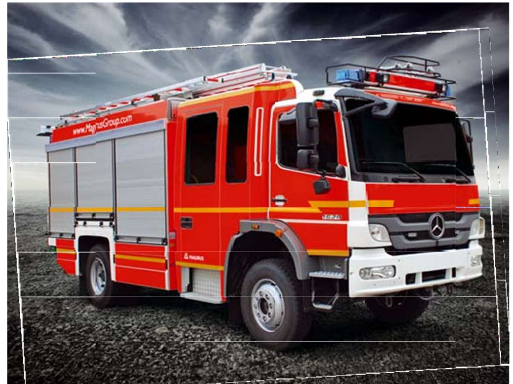
/ 2000 litre class fire-fighting vehicle on Mercedes 4x4, with MAGIRUS crew compartment in aluminium technology
