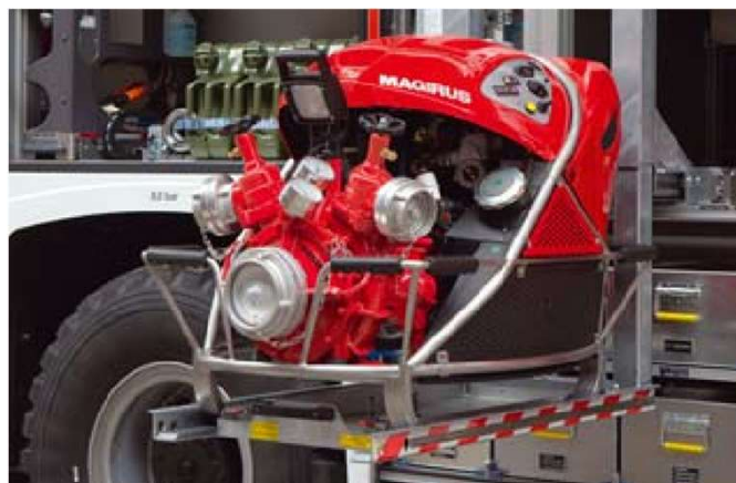
/ Lowerable fire pump storage for ergonomic removal
