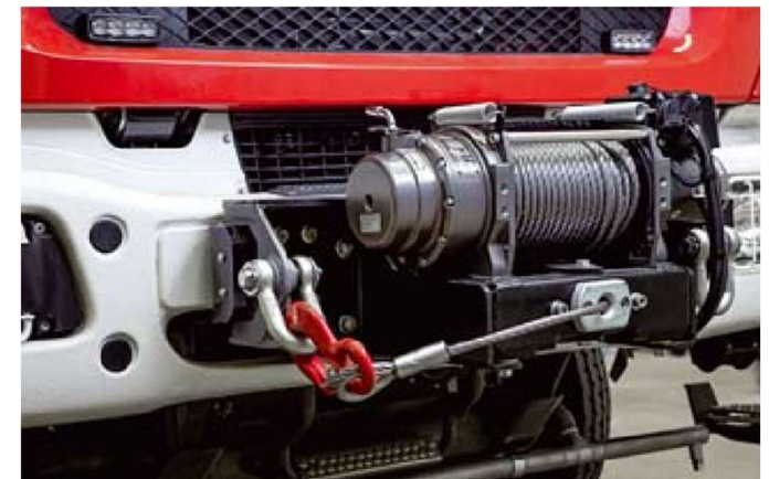
/ Front-mounted winch for technical assistance and self-removal
