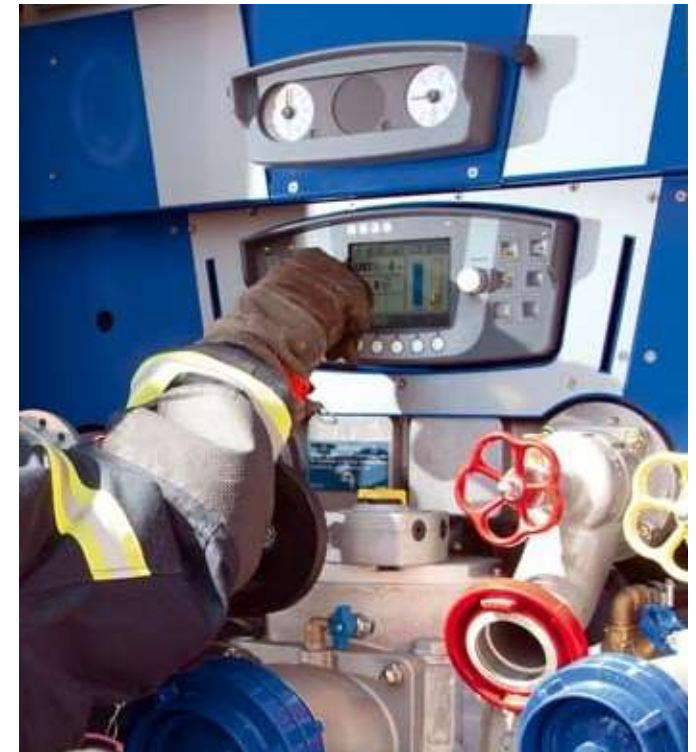
/ The rear HMI operational element is identical to the luxury version in the driver's cab. Operation while wearing gloves is not a problem. Modern – practically oriented – informative.
