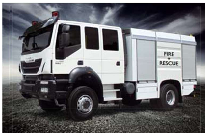
/ Multi-Purpose Vehicle with crew compartment and tank with 4,000 litres
