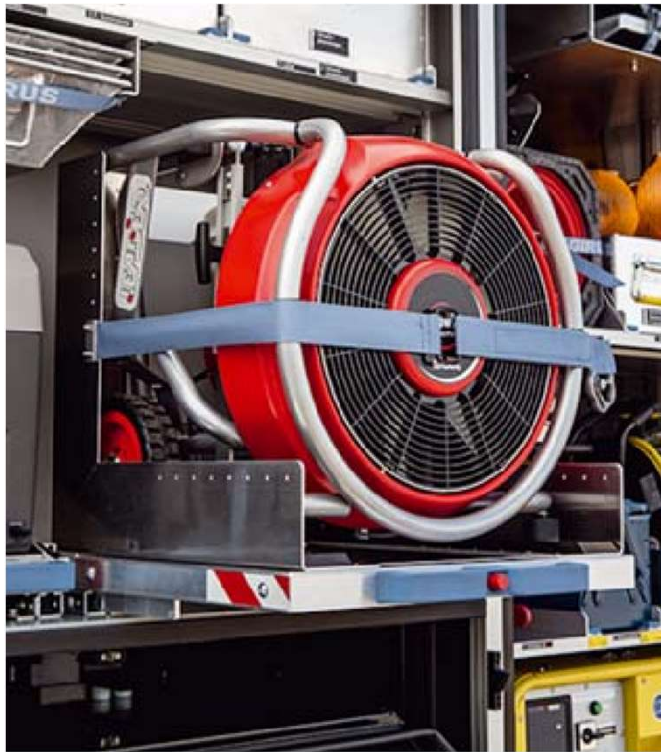
/ Heavy-duty pull-out shelves ensure optimum storage and energy-saving removal of mobile equipment units, e.g. ventilators or hydraulic rescue equipment.
