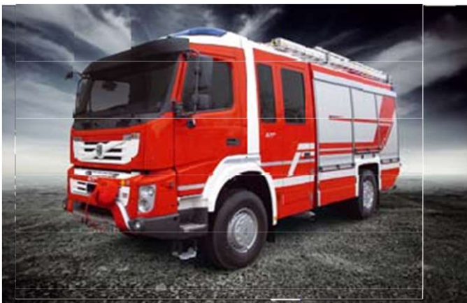
/ Customized Tank pumper with crew compartment 1+8
