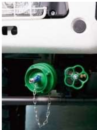
/ Front pressure outlet or roof monitor for individual emission of extinguishing agent
