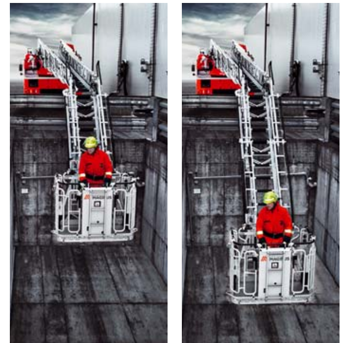
/ Penetration depth of an articulated arm turntable ladder and an articulated arm turntable ladder with telescope in comparison (left to right).
