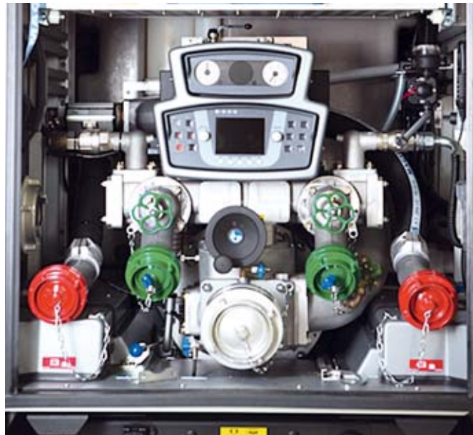
/ This variant features all the advantages of modern HMI control, but is not shielded. All components are visible and easily accessible.
