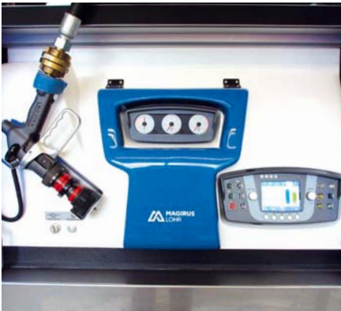
/ As an alternative the pump space can be completely shielded – here we see the Austrian variant with high-pressure quick attack. Input and output lines are located on the side or below the pump space.
