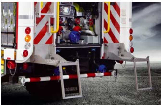
/ Double standing stations at rear for monitoring hose storage while driving
