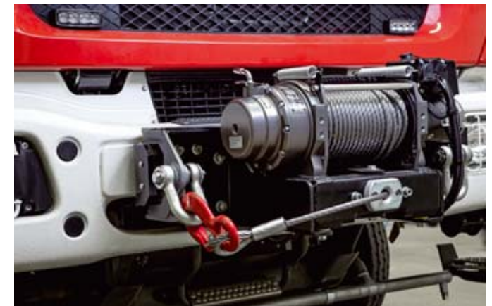
Front-mounted winch for technical assistance and self-removal
