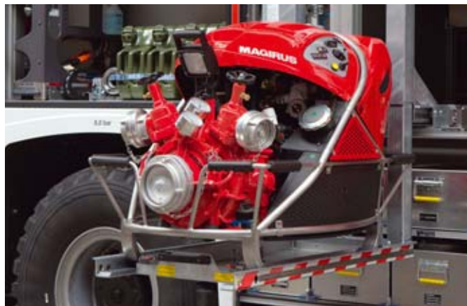
Lowerable fire pump storage for ergonomic removal
