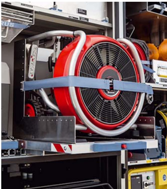
✓ Heavy-duty pull-out shelves ensure optimum storage and energy-saving removal of mobile equipment units, e.g. ventilators or hydraulic rescue equipment.
