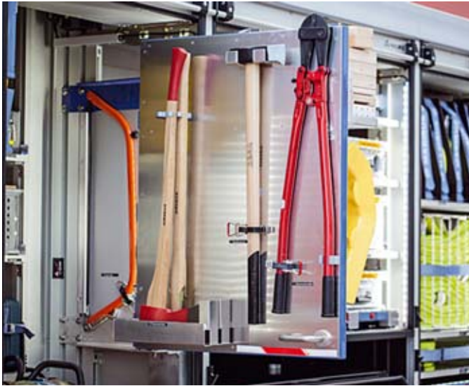
/ Accessible from two sides, the swing panel is easy to use and can be securely locked.
