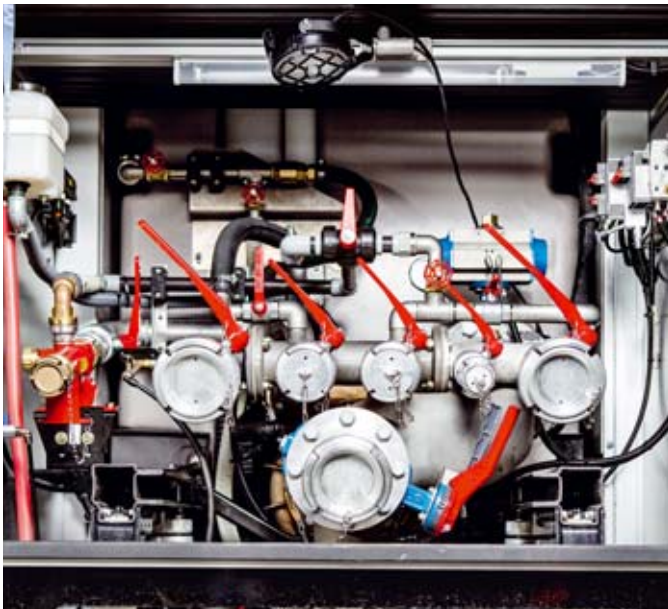
/ The version of the pump control stand in the rear of the vehicle is defined in accordance with your individual demands and specifications. The basic version has intentionally simple analogue control.
