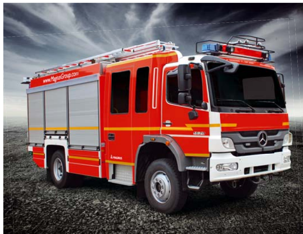
/ 2000 litre class fire-fighting vehicle on Mercedes 4x4, with MAGIRUS crew compartment in aluminium technology
