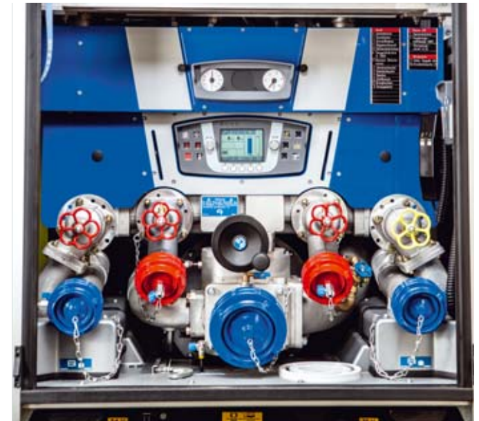
/ Partial shielding of the pump space results in a modern, orderly appearance. The connections and hand valves are open and easily accessible.
