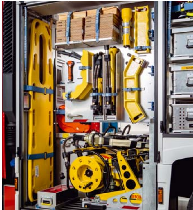
/ All equipment necessary for technical initial response is mounted on a swing panel: at eye level, clearly visible, ergonomic, efficient.
